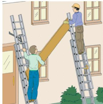
Rest the first end of the plank on the ladder jack and hold it in place while the helper brings up the second end. The first end juts over the jack as the second end comes up.
